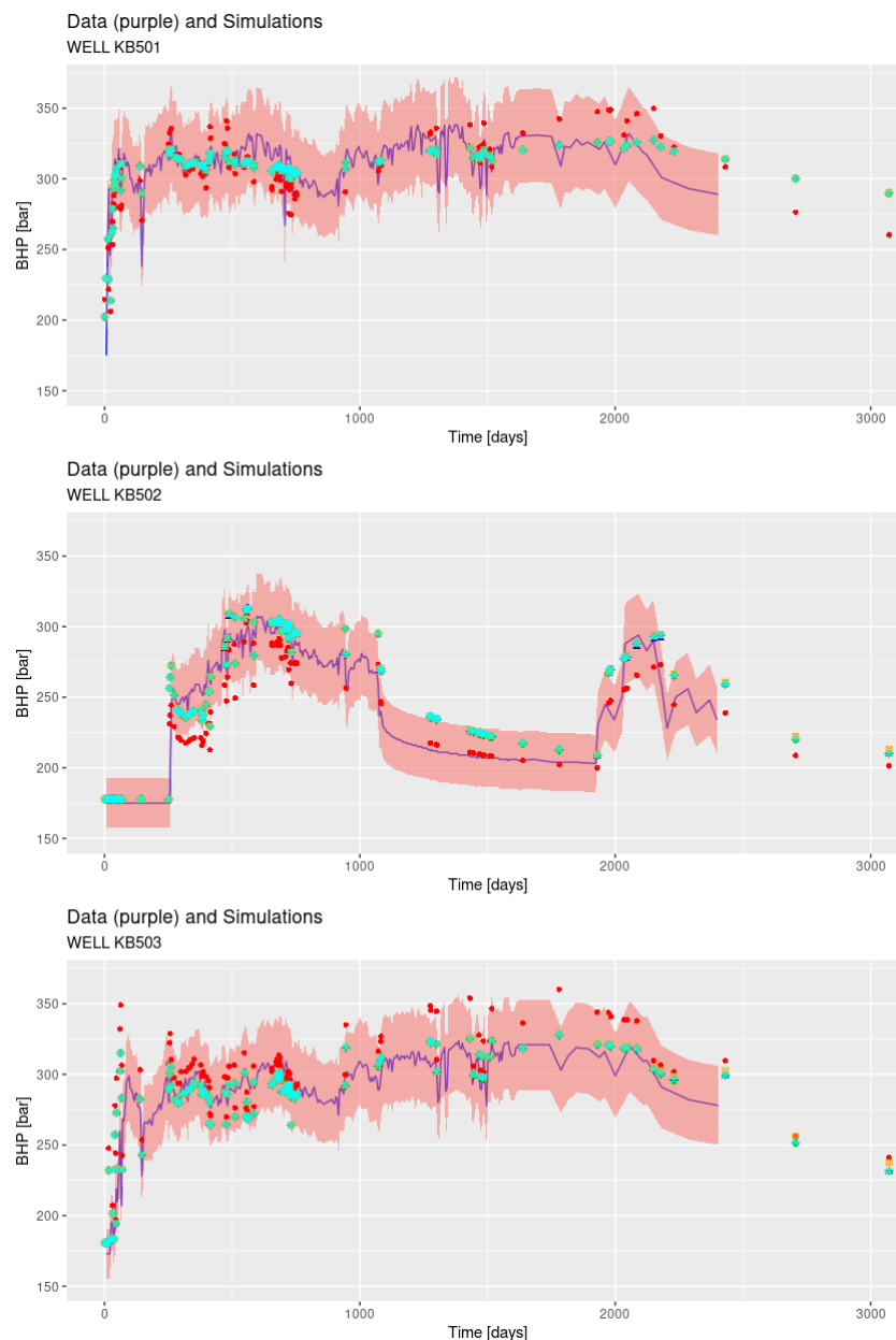
Figure 27 : BHP results from field data (purple with an uncertainty of +/- 10% (pink area)) and simulations with calibrated sensitive parameters from the first optimization (red, C_{pfs\_reserv\_kb501} and C_{pfs\_reserv\_kb503} = 2e-3 \text{ bar}^{-1} and C_{pfs\_reserv\_kb502} = 6e-3 \text{ bar}^{-1} and permeability multipliers) and from the second optimization (OF2, C_{pfs\_reserv\_kb501} and C_{pfs\_reserv\_kb503} = 1e-3 \text{ bar}^{-1} and C_{pfs\_reserv\_kb502} = 4e-3 \text{ bar}^{-1} and permeability multipliers) with dynamic permeability (green and yellow).
