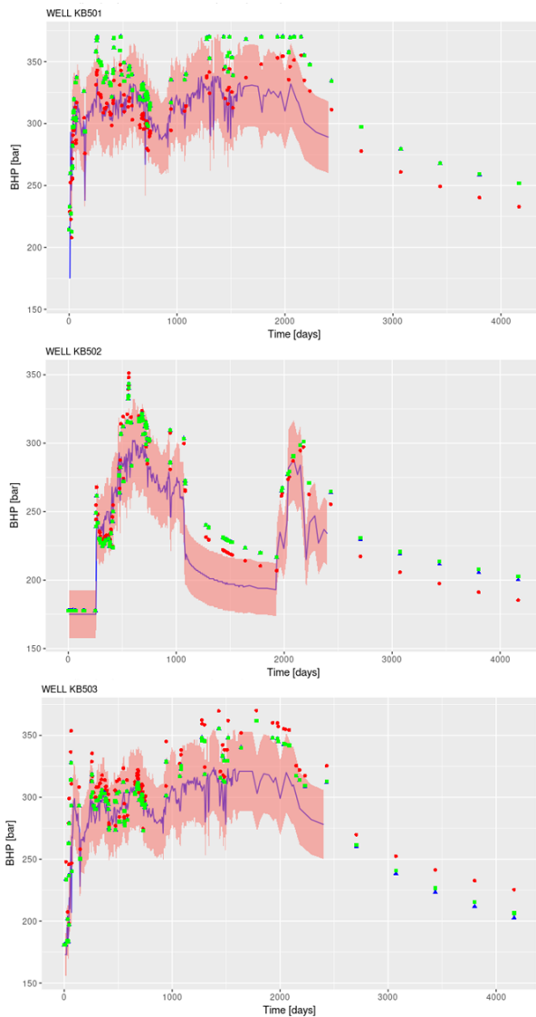
Figure 22 : Comparison of BHP results at KB501, KB502 and KB503 wells for different simulated scenarios (well blocks, pore compressibility and production rates). The purple line refers to field data with an uncertainty of +/- 10% (pink area). Red squares are results from the base case.
